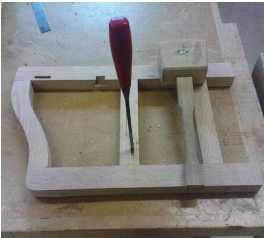
Here we can see the mortise and tenon joints for the (shelf) rails being made in one of the sides.
