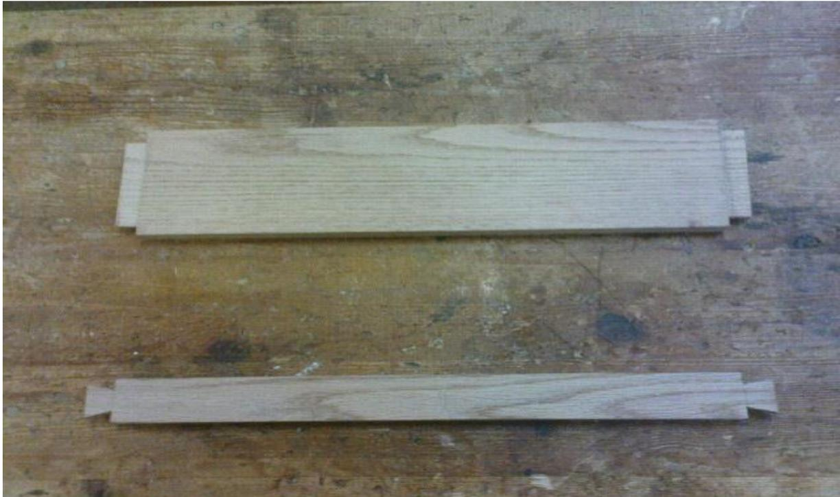
Here we can see the mortise and tenon and dovetail joints at the ends of the back rails.
