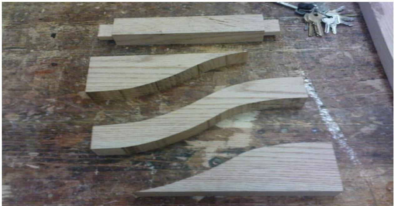
Here we can see the top curve cut out for one of the sides.
