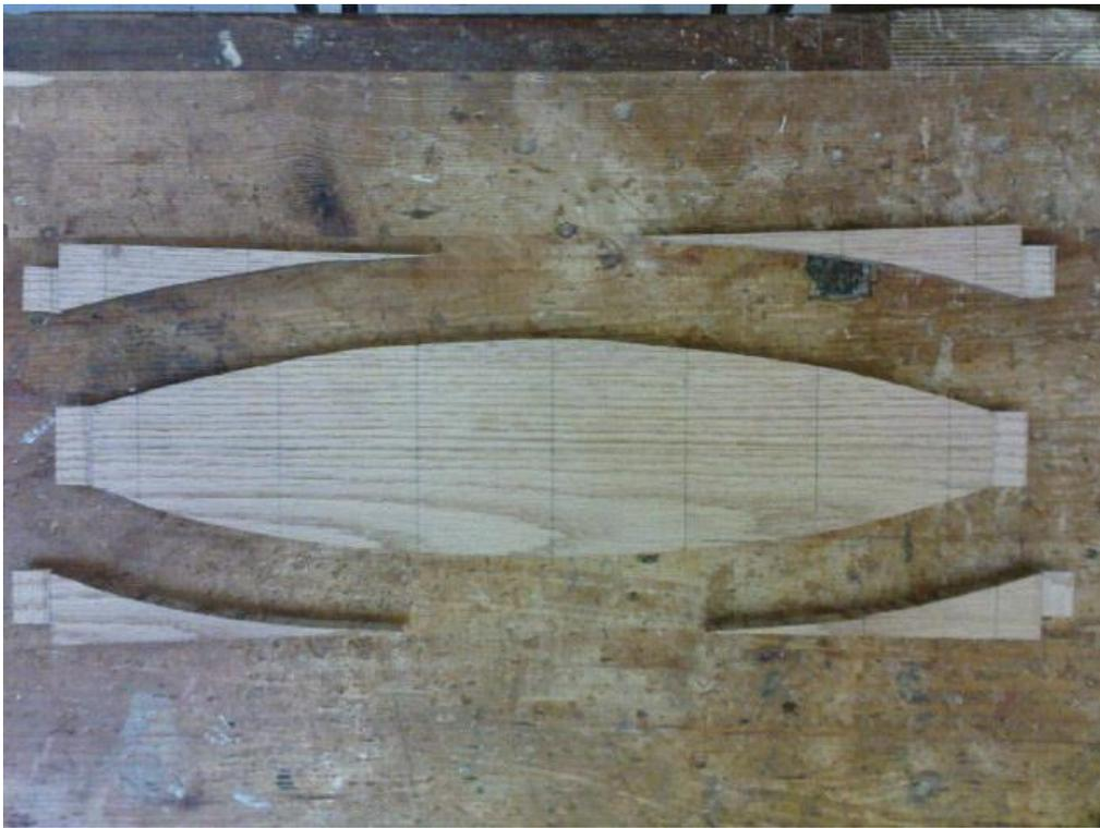
Here we can see the curve cut out on the top back rail.
