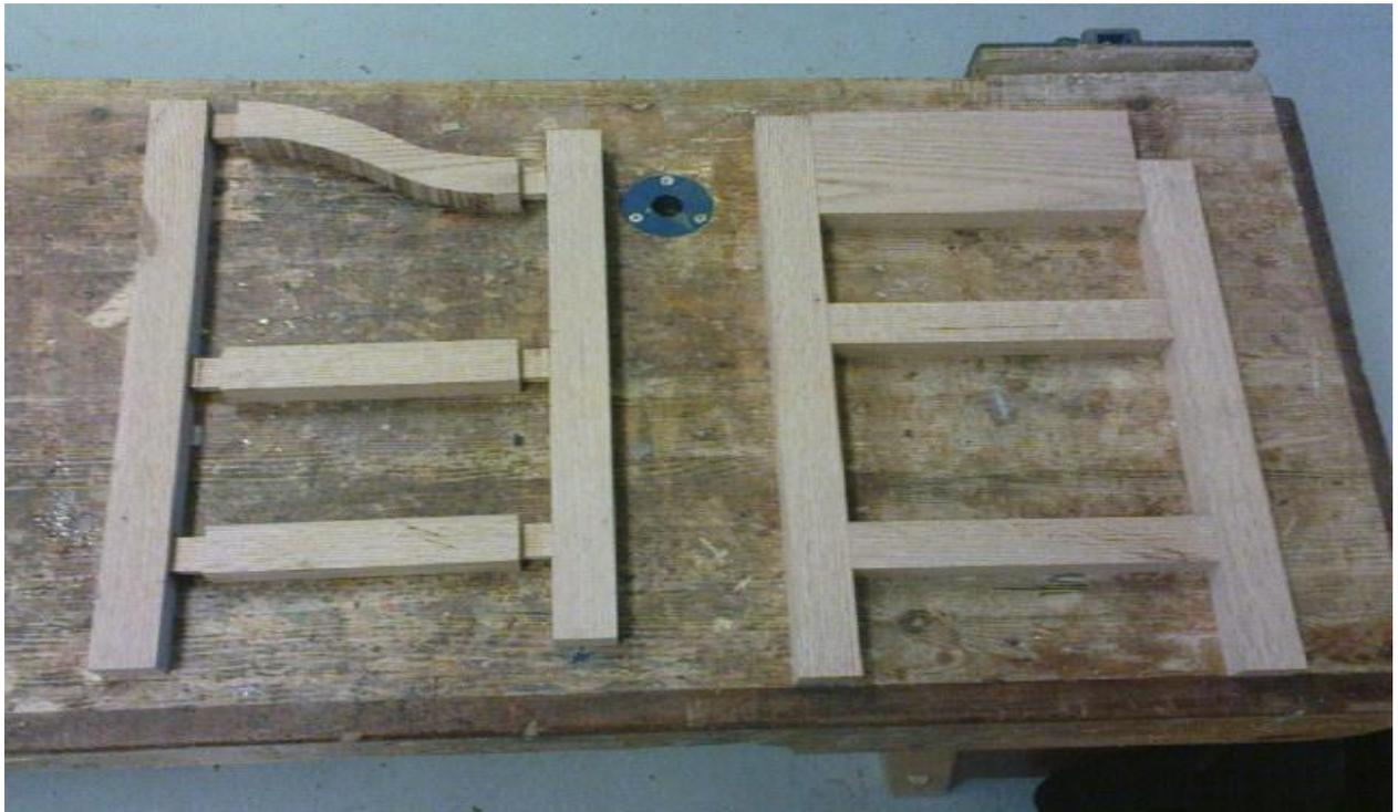
Here we can see the mortise and tenon joints for the sides.
