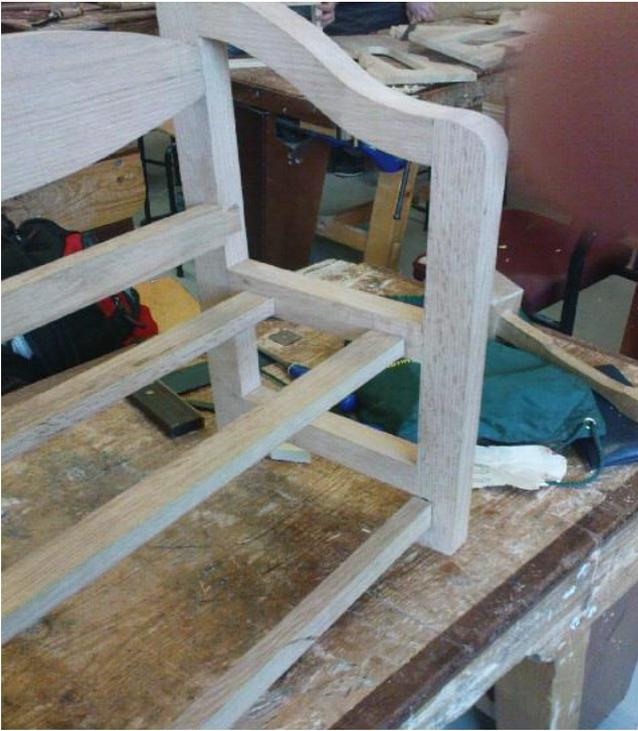
Here we can see the (shelf) rails joined onto the sides.
